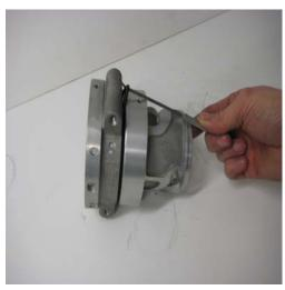
If necessary change O-ring (pos.21) for dust –protection. Use grease on the new O-ring.
