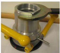
Place the swivel sleeve over the coupling body and screw in the swivel sleeve.
