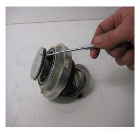
Change the O-ring (pos.3) on the piston. Use grease on the new O-ring. Make sure that the O-ring doesn't get twisted when mounting.
