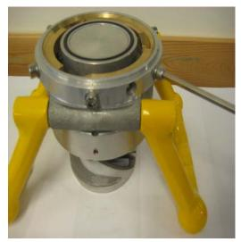
Unscrew the bolts and take out the coupling ring.
