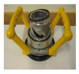
Change the Teflon® ring (pos.25) on the top of the coupling body.
