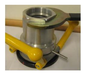
Mark the position of swivel sleeve against swivel ring with an Ø8 mm pin.
