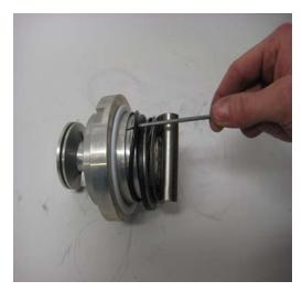
Remove and change O-ring (pos. 8) on the driving plate back side. Use grease on O-ring.
