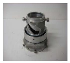
Assemble the two shafts for the piston guide.
