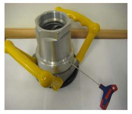
Use Loctite® 243 and screw the lock screw into the swivel ring without any force! Risk to deform the ball bearing!
