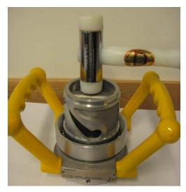
Remove the driving plate packet from the coupling body.
