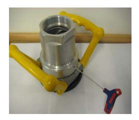
Begin with unscrewing and remove the lock screw from the swivel ring.
