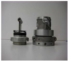
Before the coupling body places on the driving plate packet, make sure that the part where the upper cam curve ends, shall be placed exactly over one roll, and the heel on the driving plate packet should be placed under the hole for the shaft.
