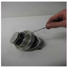
Change the O-ring (pos.6) on the driving plate front side. Use grease on O-ring.
